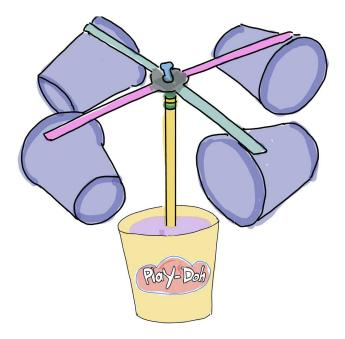
d. If you prefer, you can hold the anemometer in your hand when you are measuring wind speed.
