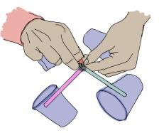
c. Insert the pin into the eraser of the pencil. This will create the axle and provide something to help keep the anemometer attached to the base.
