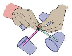
c. Insert the pin into the eraser of the pencil. This will create the axle and provide something to help keep the anemometer attached to the base.
